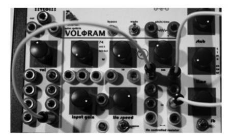
the 1-st one has 2 inputs and it can be used as crossfader / mixer / volume control
