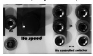
it can be used as independent sound source, modulation source or it can control other connections via "LFO controlled switcher" (resistor on some versions)
